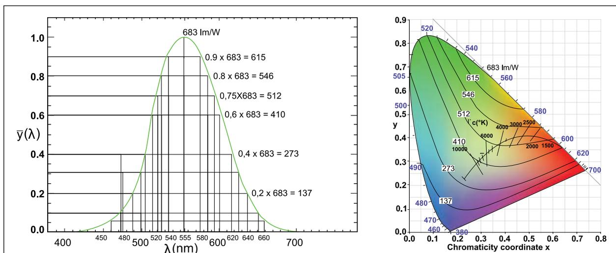
Phosphor conversion technology is based on blue photons at 440 to 450 nm which are converted to visual light in the range of 500 to 620 nm. The short wavelength high energetic 'blue' photon with a band gap of 3.7 eV hits a phosphor particle which emits in return a lower energetic Photon of 3 eV and longer wavelength. This collision results in 20% energy loss, the so called Stokes shift, which can
